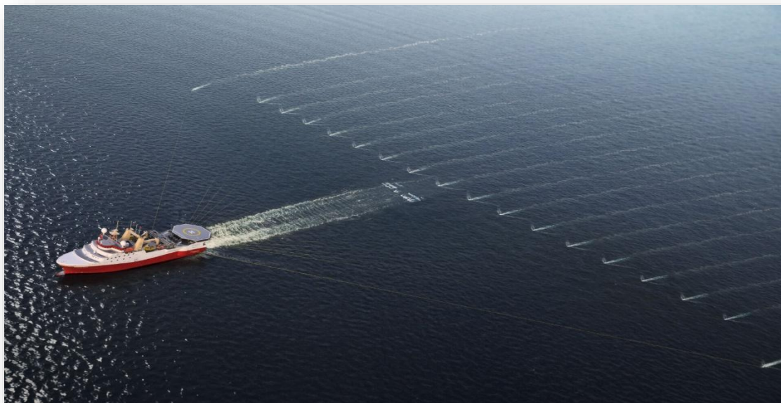
There is much rigging happening here to keep the cable spacing even. However, it is managed, and the paravanes are working hard.
