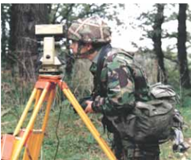
Total Station comprising theodolite, EDM and GPS functions
