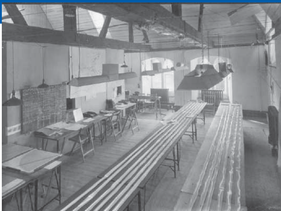
Operations room in England. Four films are laid out for reading on the tables, each film looped in a stretched "S" with two hairpin bends. The films were fed up from the recorder room below through slots in the floor and the wooden shafts seen at the far end of the tables. The bearings and elevations computed from the film readings were passed through the hatches in the wall on the left to the dark room housing the plotter.
