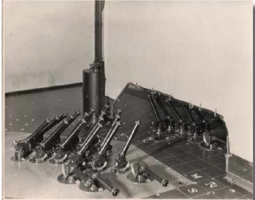
Three-dimensional plotter set with bearings and elevations of rays pointing to origins of supersonic boom reaching microphones of lattice in England. The vertical screen was pivoted on a vertical spindle placed on the map grid location of the point of burst obtained by cross-observation by flash-spotting posts. In this instance the burst was in north-east London. The screen was rotated until a trajectory descending to the point of burst was formed by the faint points of light seen on the tracing paper at the intersections of the rays with the screen. The "searchlights" not set were spares not currently in use.
