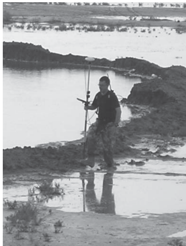
Conducting a drainage stability survey with GPS at Basrah Ai.
