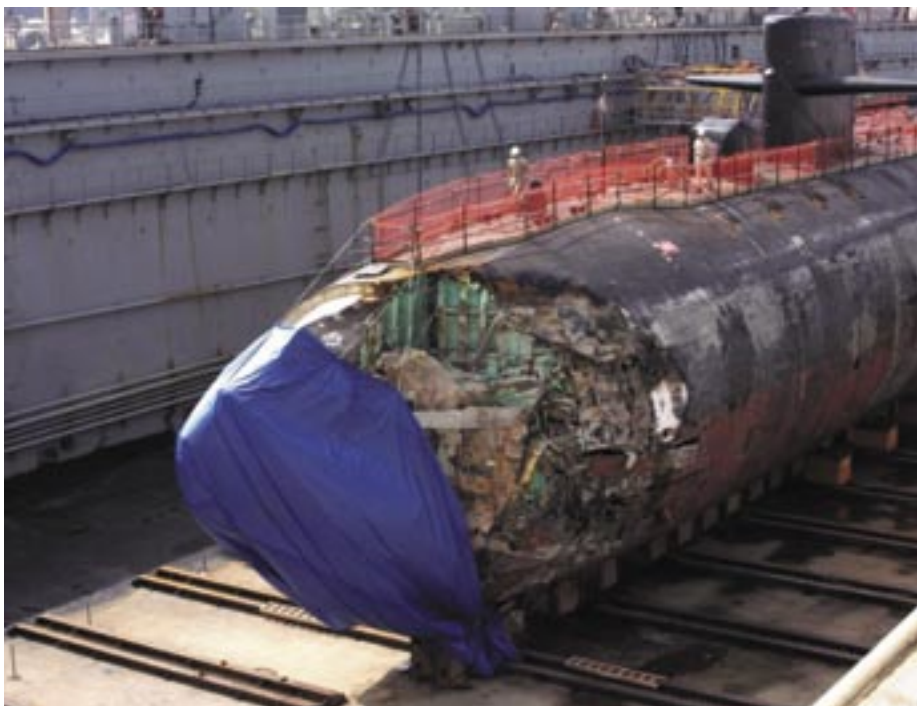
US Submarine San Francisco which hit a Sea Mount at 28 knots. The chart showing the sea mount was on board but not available to the navigator at the time of the accident.
