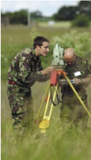
42 Engineer Regiment (Geographic) soldiers using an Electronic Total Station
